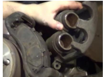
Adjust the reset plate distance and insert the tool into the caliper.
