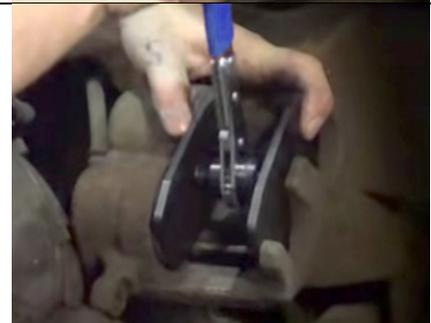
Switch the direction of the ratched and pre-load the tool in the brake caliper. Pay attention to the correct position of the tool during the pre-load..
