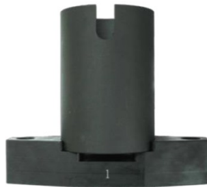
Tool installation for disassembly of silent block
