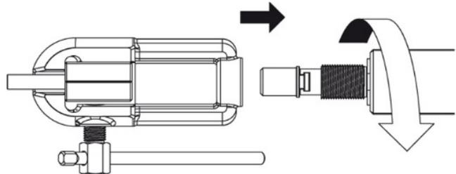
13. Then loosen the tightening bar and remove the tube. It should look something like the sketch below.
