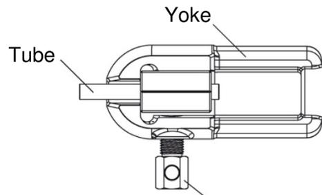
Securely fasten die by turning fixing screw clockwise with your hands.
