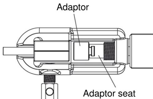
6. Begin squeezing the lever and continue until the edge of the adapter meets the die.
