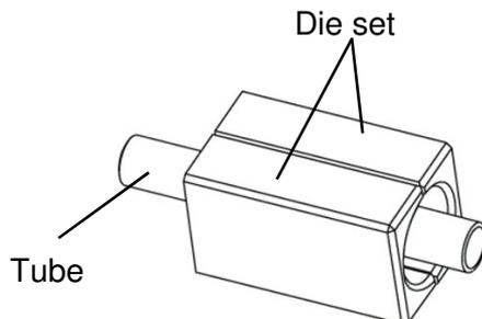
2. Insert and tighten the dies and tubing into the yoke
