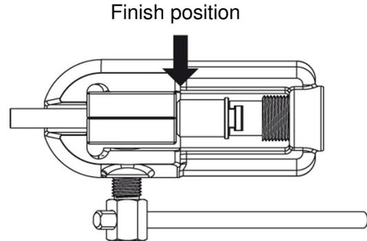
11. Open the relief valve 1/2-round, than close tightly.
