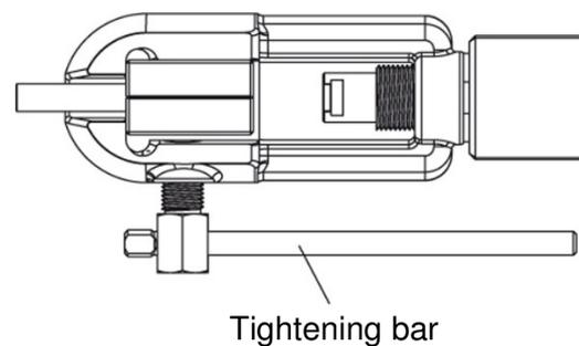
9. Rotate the tool counter-clockwise 3-round to place the adapter that you want to operate and rotate clockwise until it stops.
