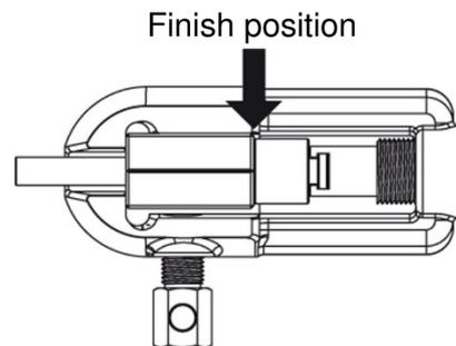
7. Open the relief valve to fully recess piston, then close tightly and remove the OP0 adapter.
