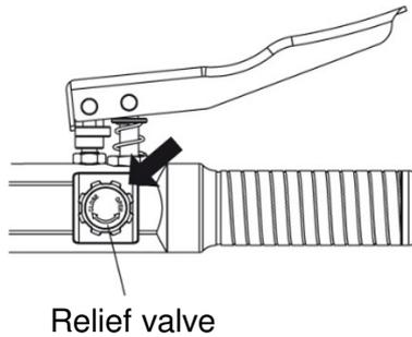
4. Grasp the handle and rotate the hydraulic cylinder clockwise until it stops.
